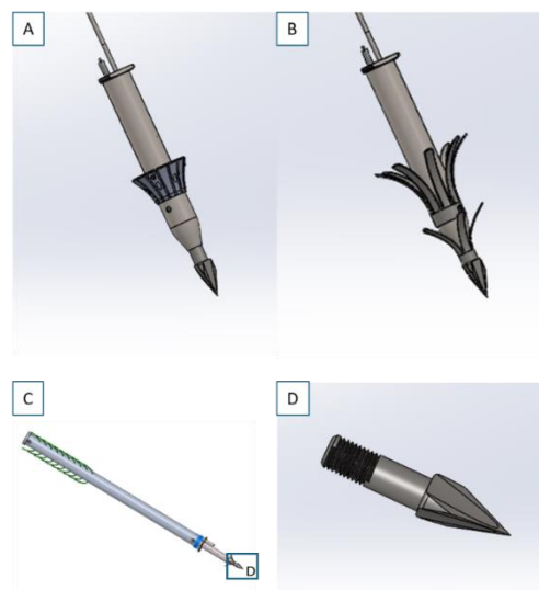
Figure 3. New design for MINTAG tags to be deployed in the summer of 2024, showing the variant with the retention cone (A) and the petal configuration (B), as well as the overall view of the improved carrier (C) and the new tip design (D).
