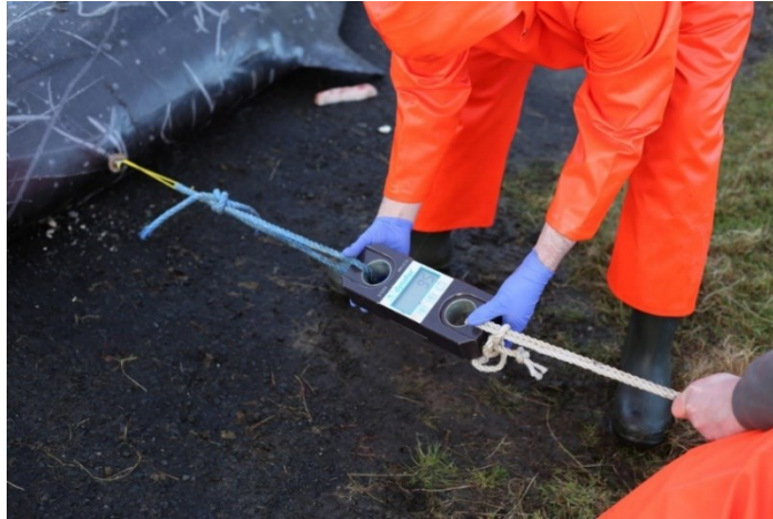
Figure A3.2. Testing the pull (kg) needed to extract the tag from the whale body
