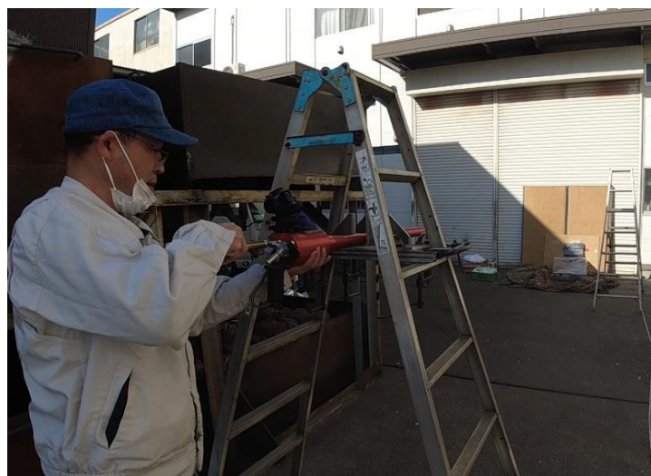
Figure A3.3. Shooting scene with the target of blubber and grass mats (7m in distance)
