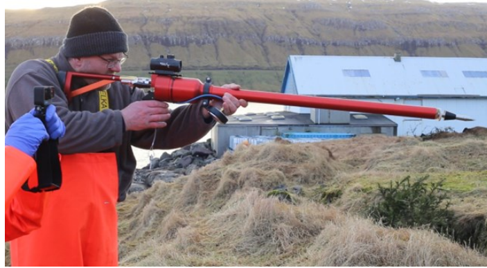
Figure 3. ARTS gun for tagging whales provided by the project and used in the Faroes test.
