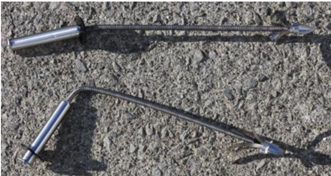
Photo shots 3.1 and 3.2. Both shots (3.1 above and 3.2 below) resulted in a bended shaft
